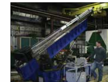
Convertible Test System 20,000 lb load - 100° CC
