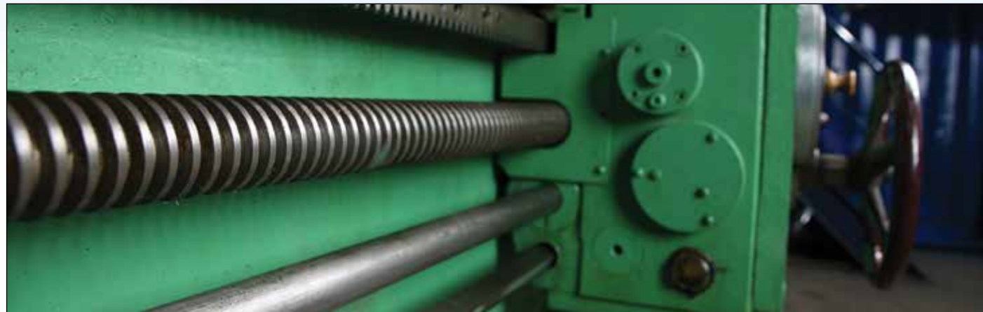
Nook acme screw used in a manual lathe
