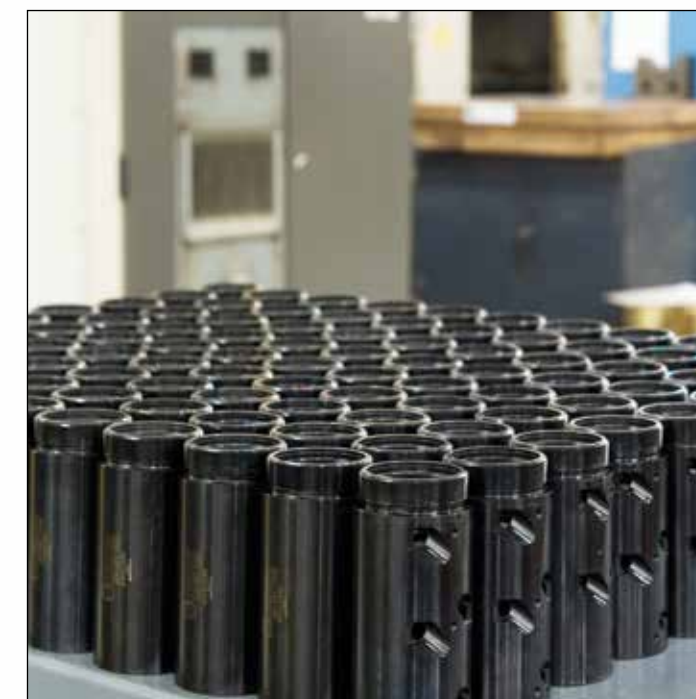
Nook 2.00" diameter ball nuts
